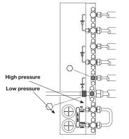
**H** Tighten connections using a spanner and a torque wrench; apply specified torque (see table).
