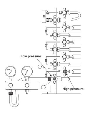
**B** Turn on the unit's operating switch and start cooling operation. When the low-pressure gauge reading falls to 1 to 0,5 Kg/cm<sup>2</sup>, close the wide tube valve and then quickly turn off the unit.
