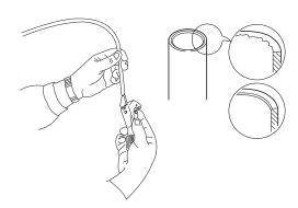
F Insert flare nuts removed from the units, than make a flare at the end of copper tubes.
