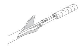
Remove caps from service valves of both tubes. Then start vacuum pump and let it run for the time indicated in the table (vacuum 10 mm Hg abs.).
