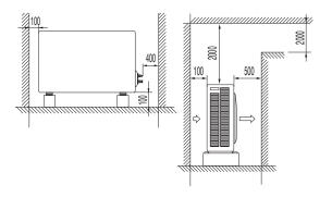
B Heat pump version. Use, if necessary, the accessories supplied.
