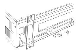
Remove the side cover, then connect the power line and interconnecting wires to outdoor unit on the terminal strip and secure them with clamps.
