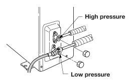
Tighten connections using a spanner and a torque wrench; apply specified torque (see table).
