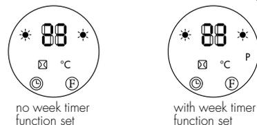
Press the + or – buttons to set the temperature. When this function is active, if the room temperature drops by 5-10 °C in less than 10 minutes, the fan heater stops operating and switches to stand-by mode.
