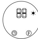
In COMFORT heating mode (2000 W) the LED display is the following:
