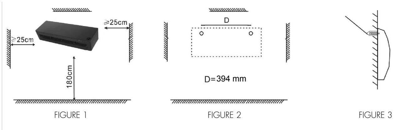
3. Insert the Fischer screw plugs into the holes and tighten the screws provided.
