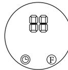
In ECO heating mode (1100 W) the LED display is the following:
