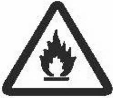
Appliance is filled with flammable gas R290.
