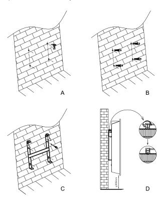
Make sure that the convector is placed at least 30 cm from the floor and that the distance from walls and objects is respected, as indicated in the figure below:
