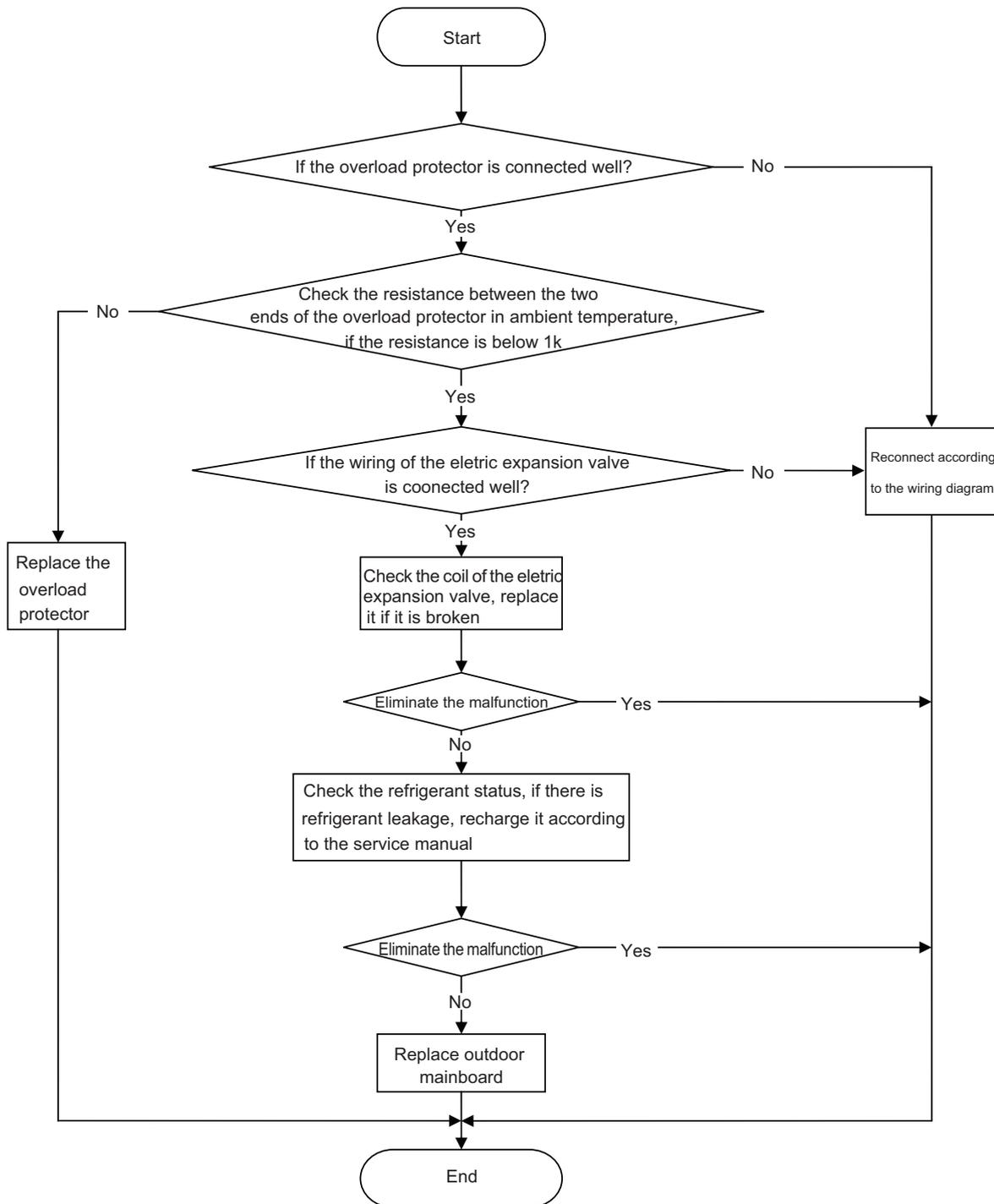
Note: the detection method of the coil of the electric expansion valve: there is five pieces of coil of the electric expansion valve, the resistance of one of them (the leftmost or the rightmost one) is almost the same as the resistance of other terminal (within  $100 \Omega$ ). Judge the condition of the electronic expansion valve through detecting these resistance.
