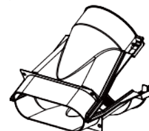
End fitting for window, supplied into 2 parts to be joined with 2 tabs that fit together. (2)
